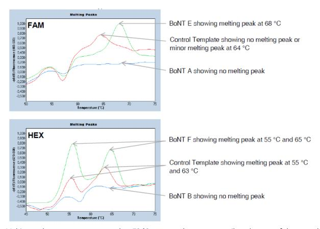
Melting peak temperatures greater than 70 °C can occur but are not attributed to one of the target botulinum neurotoxin types and can safely be ignored.
